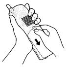
2 Replace the old battery with a new one, and close the cover (see page 12 for battery installation).
